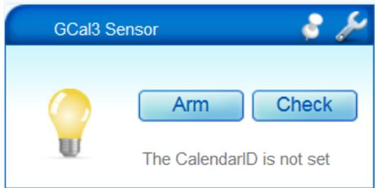
Note that the 'Arm' button is a toggle and will switch between armed and bypassed. Prior versions had separate 'Arm' and 'Bypass' buttons.
